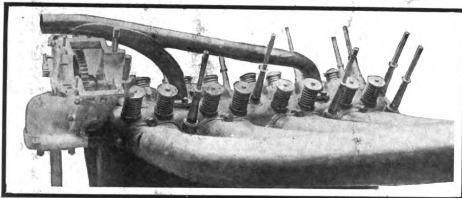
Fig. 9—Top of cylinder casting, showing studs to anchor camshaft housings
